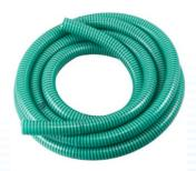
Pneumics suction and delivery hoses have proper and adequate re-inforcement which is secured by proper placement of hard spirals of rigid PVC in soft walls. It is suitable for suction and delivery of saline water, light acids, alkalis and other chemicals and for conveying granules of particles of raw materials
